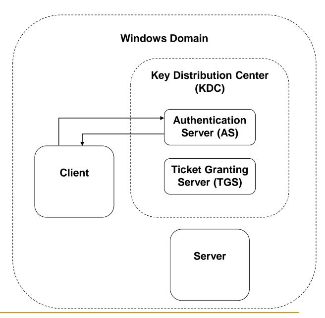
Any time the client needs to communicate with a server, it sends a message to the TGS requesting a ticket to the server
